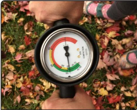
Penetrometer used to measure soil compaction.
